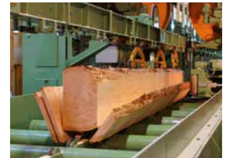
3. Sawing side boards
